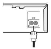
1 Plug the supplied AC power cable into the AC IN inlet and the other end into a standard household power outlet.
